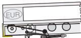
The running pallet depresses the safety separator paddle and pushes the stopper up.
