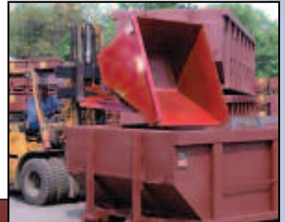
LH HOPPER DUMPING INTO CONTAINER
