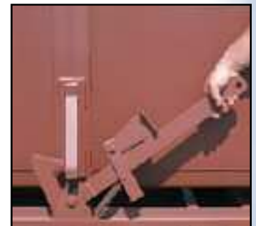
SPRING LOADED LATCH WITH REINFORCED LATCH PIN
